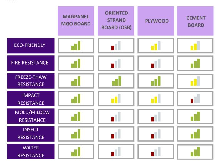
MagPanel gains its strength and resistance from very strong bonds between magnesium and oxygen atoms that form magnesium oxide crystals. It is a mineral-based green building material that will not warp, swell, or rot when exposed to water or other elements.
